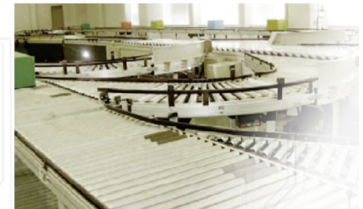
SELF PROPELLED ROLLER CONVEYOR
