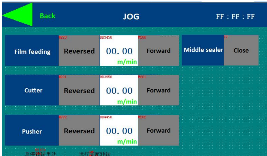
( Jog interface of belt conveyor feeding )
